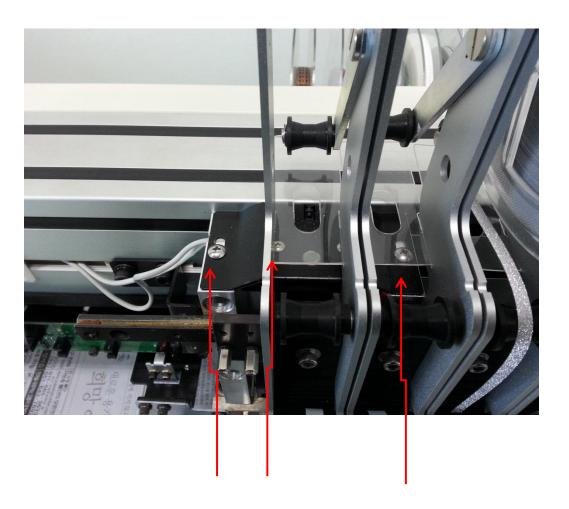
4. Unscrew these bolts and disassemble this sensor(with cover)
